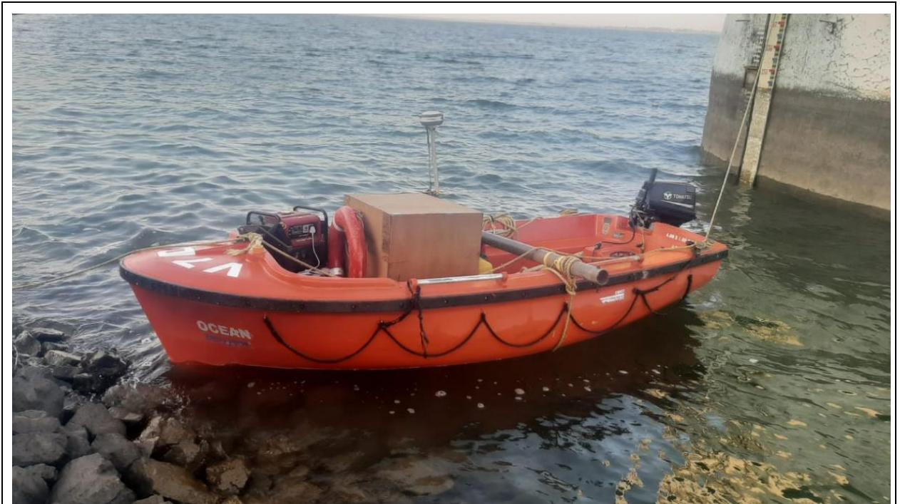
Figure 5: Survey vessel – SMB Ocean
